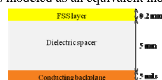
Fig.1 Dielectric profile of thin and wide band RA.
